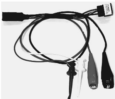
**Figure 8 Scan Tool Adapter #94020**
