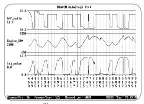
AutoGraph<sup>™</sup> allows you to view performance data graphically. Discover relationships between parameters and quickly assess the effects of your engine modifications.
