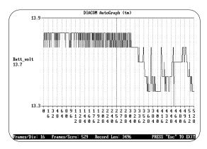
Automatic scaling of vehicle information provides the best viewing resolution and displays the details you need to zero in on elusive or intermittent problems.
