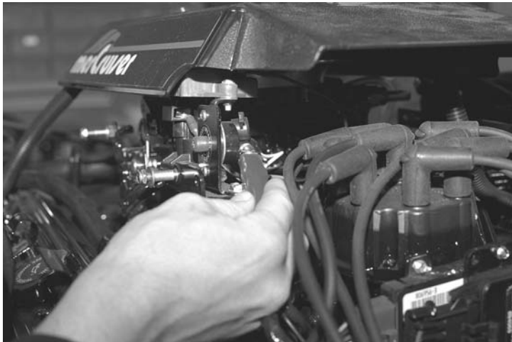
Figure 12 Circuit Breaker Terminal
